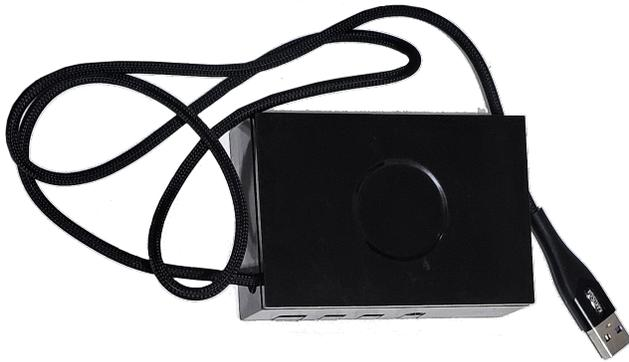
3. USB type-C to type-C cable (from Cosmostreamer box set). **It is a non-standard cable**, without a power lane (cut out 5 Volts red wire).
